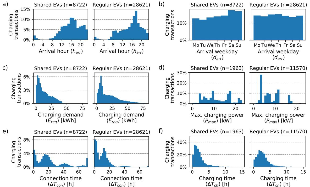
Fig. 1: Histograms comparing key charging characteristics of shared and regular EVs in the input data.
