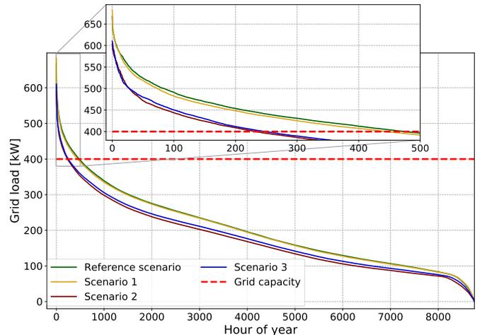
Fig. 3: Load duration curve of transformer load in the investigated grid for the four considered scenarios.
